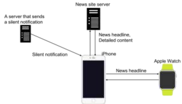
Figure 2: Overall image of smart watch cooperation PINOT information to the iPhone. The iPhone provides news information to the user and learns the user's interest from the user's behavior on the provided news information. Through learning, articles that are determined to be interested are sent by Apple Watch. Articles sent from iPhone are displayed on Apple Watch, and those that the user wanted to read are designated as “articles to be read later”.
